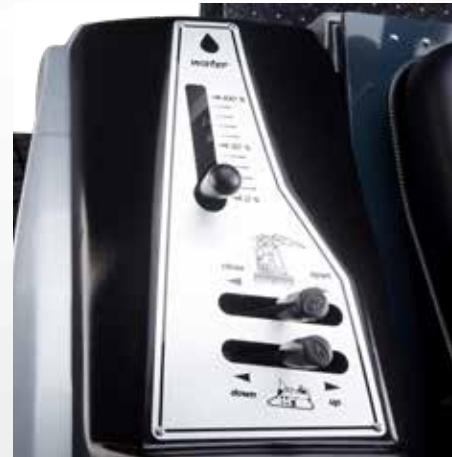
Controls for water, planing device and snow tank cover
