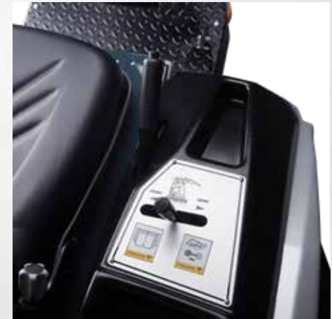
Controls for snow tank cover
